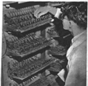
CONTAINING 1,000 TUBES, 500,000 RESISTORS, 100,000 CAPACITORS, AND 100,000 CONTACTS, THE AUTOMATICALLY CONTROLLED CALCULATING DEVICE AT HARVARD UNIVERSITY, BUILT & DISTRIBUTED FROM OTHER AUTOMATIC CALCULATING DEVICES BY THE USE OF A MEMORY-MACHINE SYSTEM.
