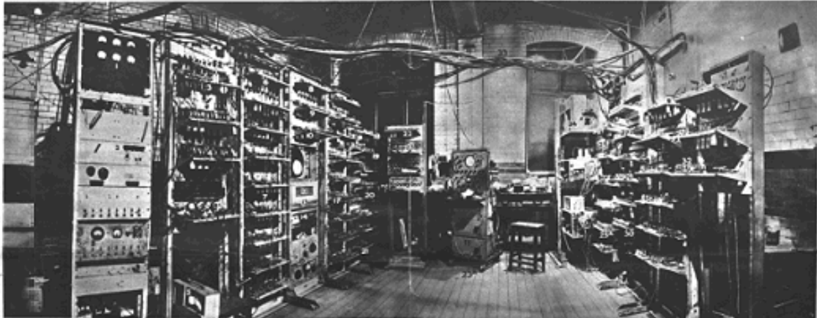
CONTAINING 1,000 TUBES, 500,000 RESISTORS, 100,000 CAPACITORS, AND 100,000 CONTACTS, THE AUTOMATICALLY CONTROLLED CALCULATING DEVICE AT HARVARD UNIVERSITY, BUILT & DISTRIBUTED FROM OTHER AUTOMATIC CALCULATING DEVICES BY THE USE OF A MEMORY-MACHINE SYSTEM.
