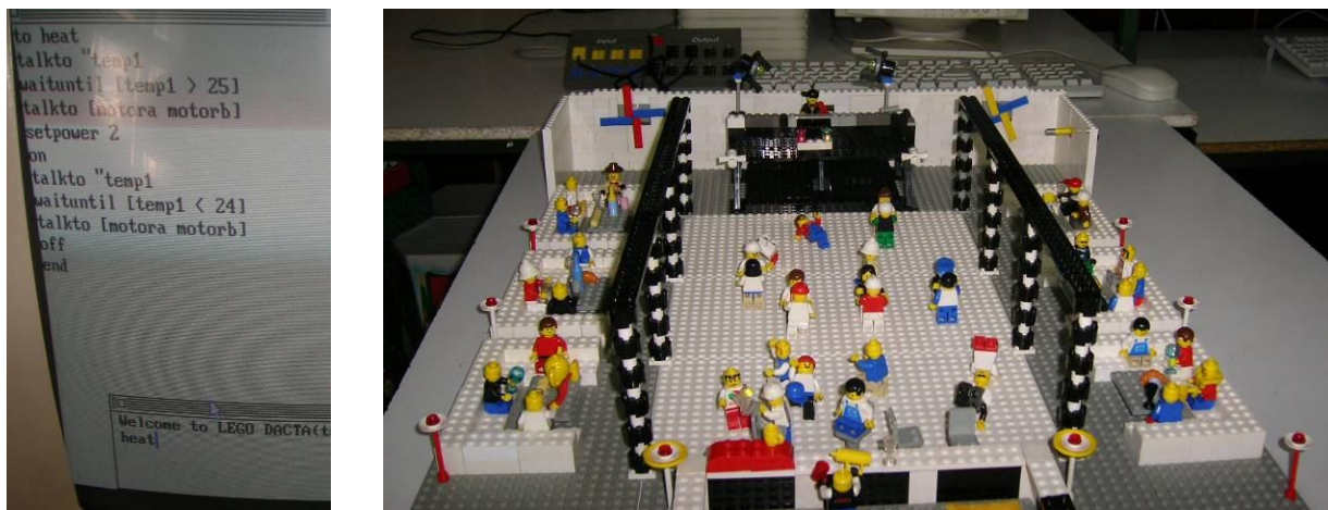
Figure 5. Ventilator control procedure for the sensor and motors, at the back of the discotheque
