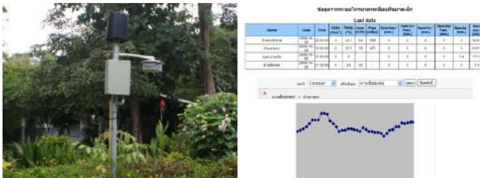
Figure 3. (Left) The weather station installed at the Ban Samkha village. (Right) The rainfall information is uploaded to a website accessible by students.
