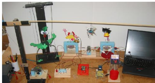
Figure 3 – Scratch Robots Construction System
