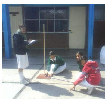
Figure 8. Measuring the angle between the sun rays and the vertical direction .
