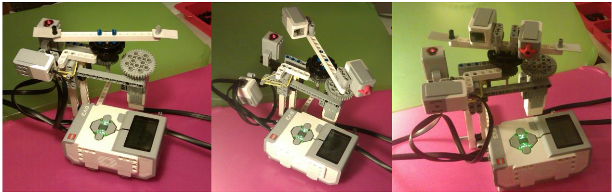
Figure 4: A physics project on rotational inertia momentum: weight distribution influences kinetic energy.
